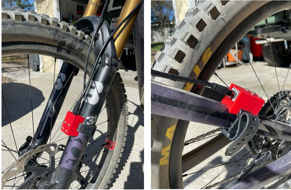
Figure 2: Accelerometers Positioned at the Fork and Seat-stay Respectively
