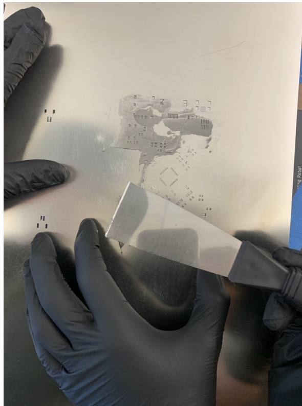
Figure 11. Applying Solder Paste Using the Stencil
