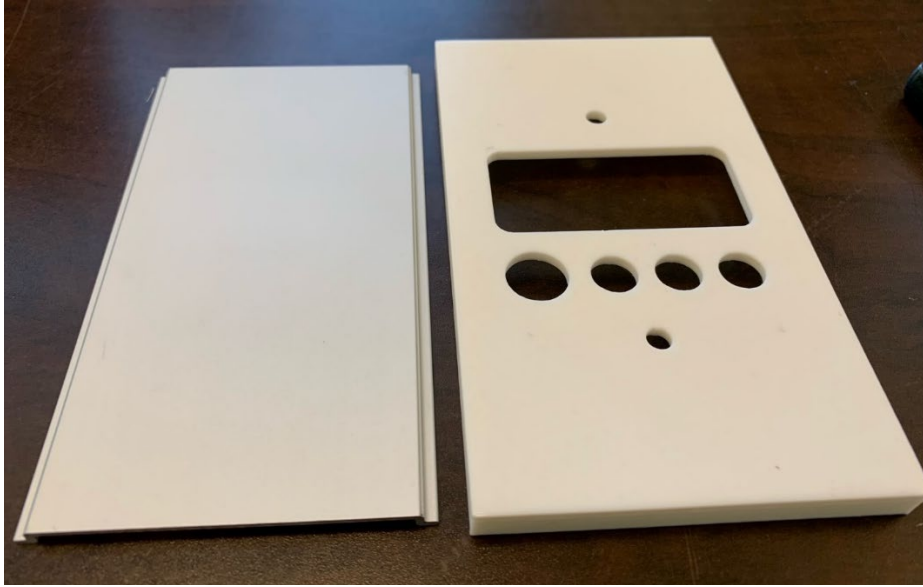
Figure 9. DAQ Housing Faceplate with 3D-Printed Manufacturing Stencil
