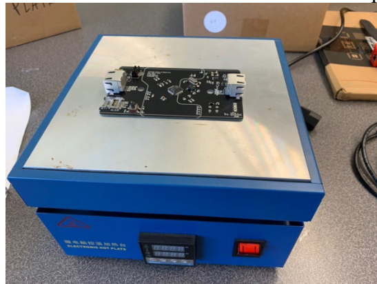
Figure 13. Using Hotplate to Simulate Reflow Oven
